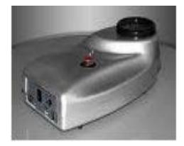
**Figure C-1:** Photograph of GDV Camera pro version 3 designed for measuring drops of liquid. There is a special syringe holder that is placed on top of the black ring which can hold a drop from a syringe just above the glass plate where the measurement is performed.
